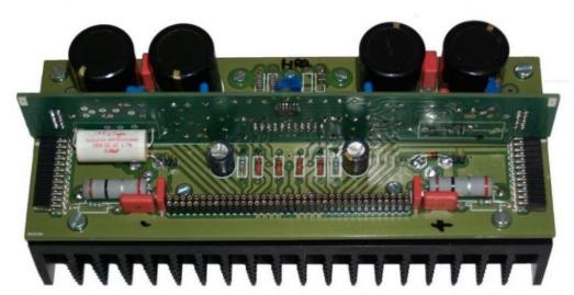
Only a combination of a VS-, and a Cs-module form a power amplifier as you are used to. So, you need both!
