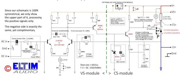
NOTE: if you always worked with power transistor based amplifiers, the function and connection of Mosfets can be confusing.
