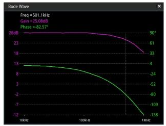
Wide audio bandwidth graph 10-100.000Hz with the marker set at 20kHz. Freq. graph straight as a ruler ±0,2dB. At this 20kHz the input to output phase error is at a minor -3°, meaning that the 3D staging (= phase!) is phenomenal, since the phase behaviour of an amplifier (and speaker) defines the 3D staging it shows. Linear (flat) = most optimal. VS-20 i.c.w. >VS-75 -3° is around 25kHz.....
